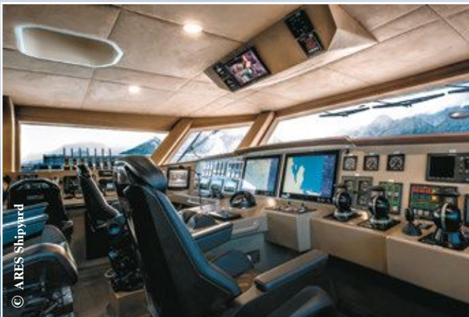
A view of the bridge on ARES 150 HERCULES. The bridge consoles of all HERCULES series boats are nearly identical. Similarly, the boats of three different sizes have many subsystems that are similar or identical, which is important in terms of logistics and manageability.
