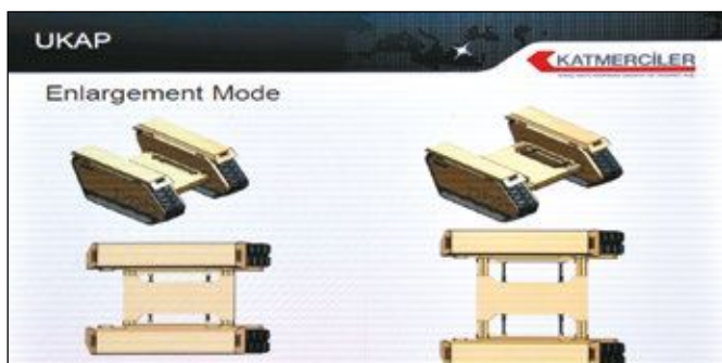
UKAP's width (left) and height (right) are both adjustable.
